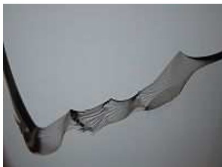
Figure 10.3: A brittle fracture in glass
