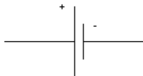
Figure 6.4 Schematic Symbol of Source of emf
